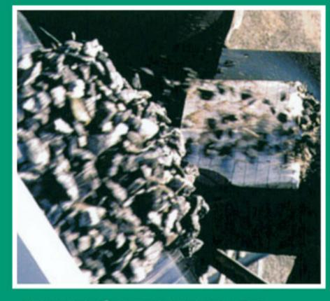
WearSpan® panel after several million tons of granite has worn through without fracture or delamination failure.
