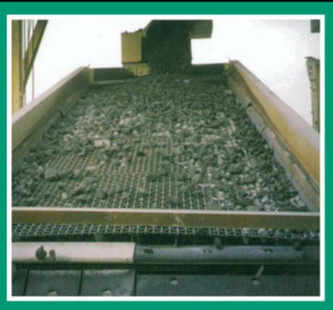
WearSpan® outlasts rubber in this screen lip liner application handling granite.
