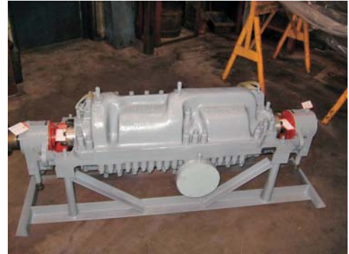
Figure 1. The 9-stage boiler feed water pump.
