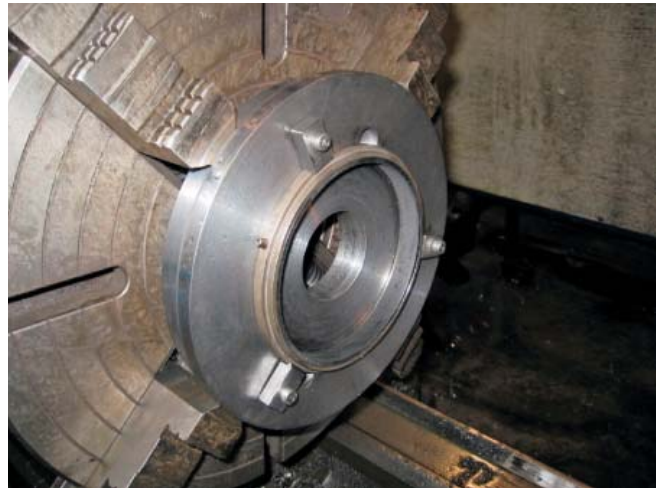
Figure 3. Composite insert in metal case ring holder.
