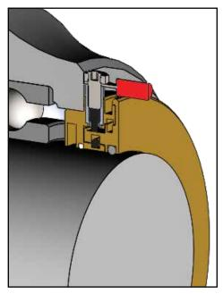
Isolated conductive filaments contacting the rotor are protected from contamination and shaft conditions, providing premium shaft grounding.
