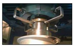
The Smart CDR can be installed with a variety of mounting configurations, including pressin, clip-on, epoxy, bolt-through, side-mount and flexbracket.
