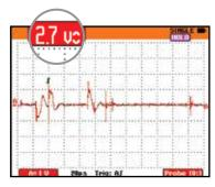
Shaft voltage with the Inpro/Seal Smart CDR
