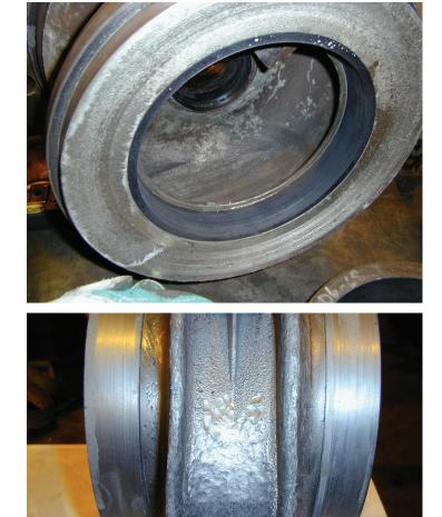
applications, however, often creates a dry-running situation. Tanks need to be emptied, light products vaporize, and sometimes debris (or a closed valve) blocks the pump suction. In these situations, metal wear components can seize and cause severe damage. Conversely, Vespel CR-6100 wear rings can survive running dry for significant periods of time, minimizing damage to pump internals. In some cases, the
